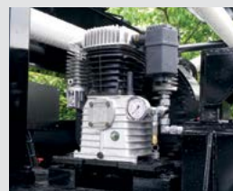
Air compressor for pipeline cleaning
