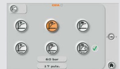
RAMPS MANAGEMENT Fully adjustable pumping ramps management
