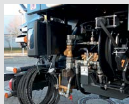
High pressure water pump
