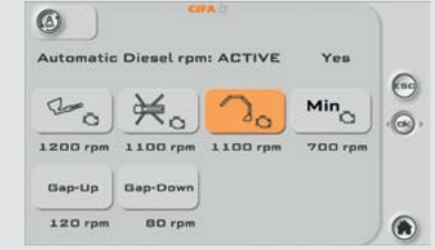
AUTO RPM Fully adjustable automatic truck RPM management
