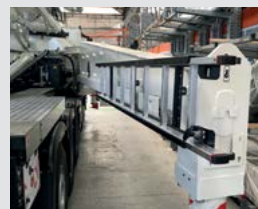
Ladder to fuel tank access
