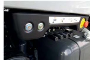
HYDRAULIC OUTRIGGERS CONTROL Hydraulic controls on both sides of truck pump. The machine emergency stop is also positioned nearby.
